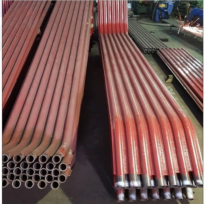
(Side & Right Wall Panel Tube Boiler)
